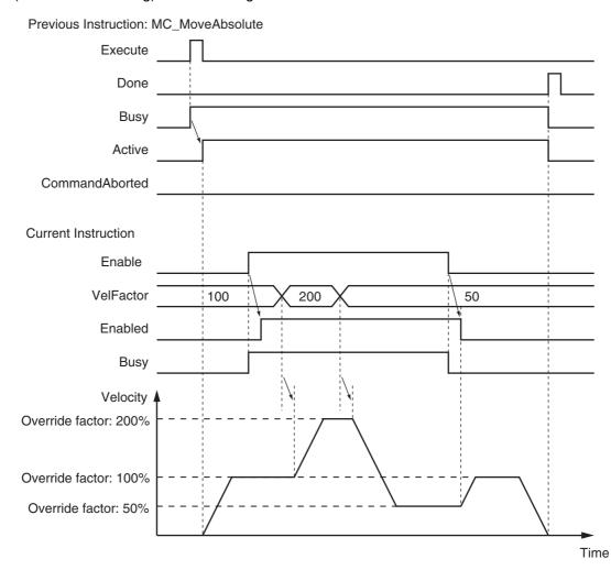
If the MC\_SetOverride instruction is disabled, the target velocity returns to an override factor of 100%.
