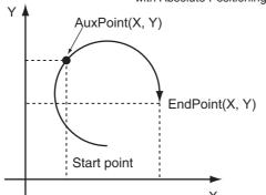
Circular Interpolation Method: Border Point Specification with Relative Positioning
