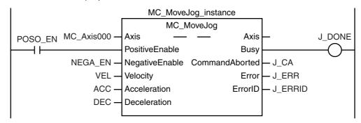
To use the master control instructions (MC and MCR) for the MC MoveJog (Jog) instruction, do not program the instructions as shown below. If you do, master control is applied only to PositiveEnable (Positive Direction Enabled), i.e., it is not applied to NegativeEnable (Negative Direction Enabled).
