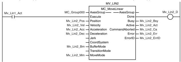
Linear interpolation (3) is executed with multi-execution of instructions after linear interpolation (1) is started.
