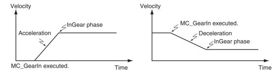
When the *Acceleration* (Acceleration Rate) or *Deceleration* (Deceleration Rate) is 0 and you execute this instruction, the axis will reach the target velocity without accelerating or decelerating.
