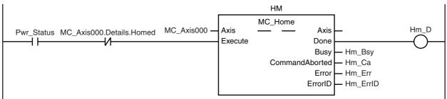
After home is defined, absolute positioning 1 is executed to move to 290.0°. The shortest way is specified for the motion direction.
