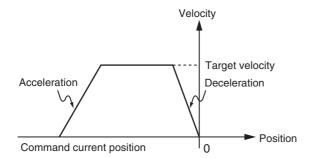
When the acceleration rate or deceleration rate is 0 and the instruction is executed, it will reach the target velocity without accelerating or decelerating.
