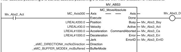
After absolute positioning 2 is started, absolute positioning 3 is started with multi-execution of instructions.
