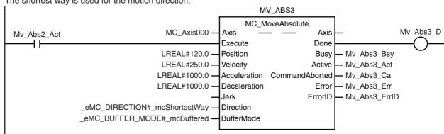
Absolute positioning 4 is executed with multi-execution of instructions to move from  $120.0^{\circ}$  to  $0.0^{\circ}$ . The shortest way is used for the motion direction.
