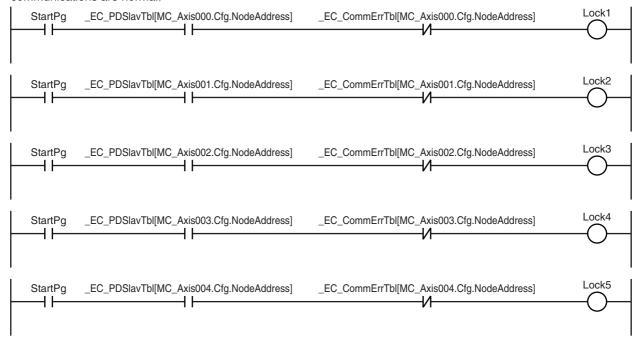
If process data communications are active, the Servo is turned ON for the axes.
