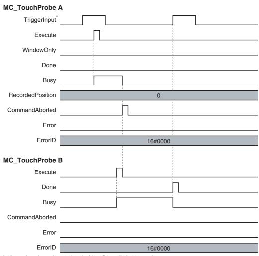
$<sup>^{\</sup>star}\,$  Here, the trigger input signal of the Servo Drive is used.
