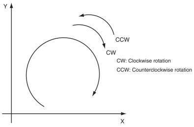
Specify the axes to use as the X axis and Y axis with CircAxes (Circular Axes). Use logical axes (axis A0 to A3) for the axes, and not axis numbers (axis 0 to 63).
