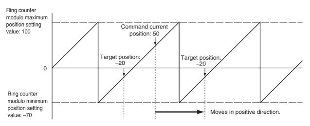
Positioning starts in the negative direction towards the target position when the negative direction is specified for *Direction*. The following chart shows an operation example when positioning starts with a command position of 50 and moves toward –20.
