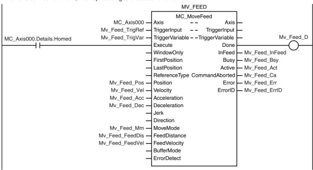
If home is defined for axis 2 and interrupt feeding is completed for axis 1, absolute positioning is performed for axis 2.
