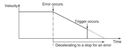
The OMRON G5-series Servo Drive executes an immediate stop when the trigger occurs. When the MC Function Module detects that the OMRON G5-series Servo Drive has stopped, it performs an immediate stop.
