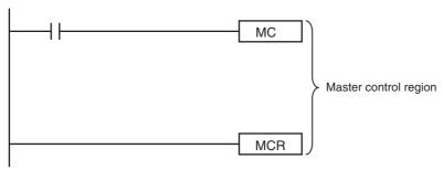
If a motion control instruction is located in the master control region, and the MC input condition is FALSE, the following will occur.
