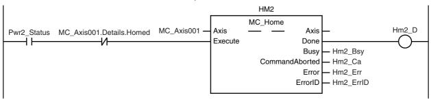
The parameters are set for interrupt feeding, absolute positioning, and high-speed homing.
