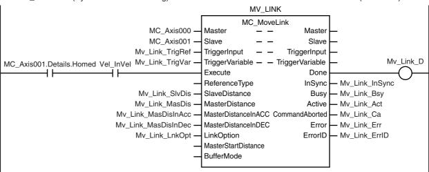
Actuator is TRUE while the axes are synchronized.
