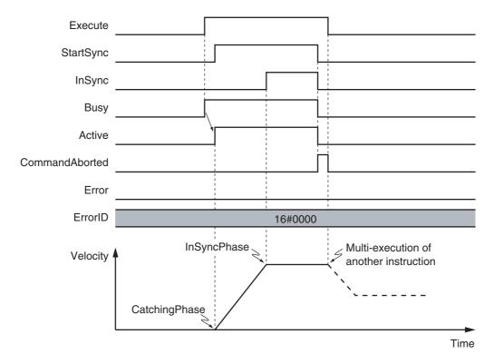
Depending on setting of the *SlaveSyncPosition*, the axis may not reach the target velocity. An example of this is shown below.
