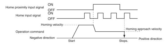
The following timing chart shows the operation when the home input detection direction is TRUE (negative direction).
