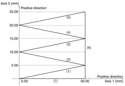
Positioning is performed using linear interpolations in the order (Axis1, Axis2) = (50.00 mm, 5.00 mm)  $\rightarrow$  (0.00 mm, 10.00 mm)  $\rightarrow$  (50.00 mm, 15.00 mm)  $\rightarrow$  (0.00 mm, 20.00 mm)  $\rightarrow$  (50.00 mm,  $25.00 \text{ mm}) \rightarrow (50.00 \text{ mm}, 0.00 \text{ mm}) \rightarrow (0.00 \text{ mm}, 0.00 \text{ mm}), \text{ then stop.}$
