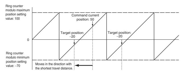
Movement is in the same direction as the current direction if the travel distance is the same in the positive and the negative direction.
