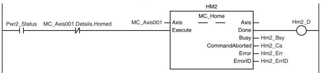
After home is defined for axis 1 and axis 2, the axes group is enabled.
