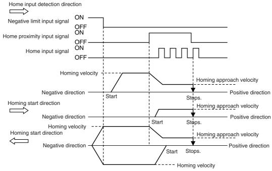
• If you start homing while the home proximity input signal is ON, the axis performs the following operation depending on the setting of the homing start direction.
