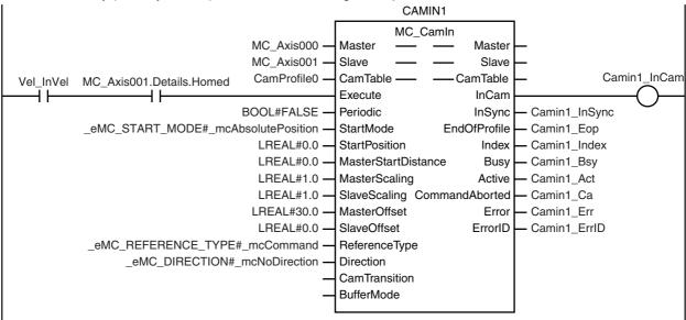
The MC\_CamIn (Start Cam Operation) instruction is executed for axis 3 (slave axis) if *Vel\_InVel* is TRUE for the MC\_MoveVelocity (Velocity Control) instruction and homing is completed for axis 3.
