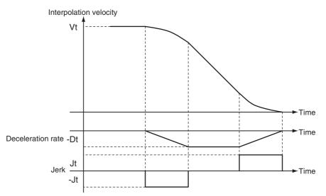
Vt: Velocity when deceleration starts, Dt: Specified deceleration rate, Jt: Specified jerk
