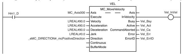
After homing is completed for axis 2 (slave axis), MC\_GearInPos (Positioning Gear Operation) is executed to start gear operation if *Vel\_InVel* of MC\_MoveVelocity is TRUE.
