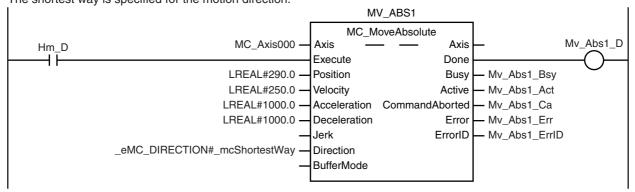
Absolute positioning 2 is executed with multi-execution of instructions to move from 290.0° to 90.0°. The shortest way is used for the motion direction.
