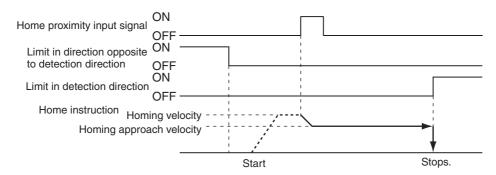
An error occurs and the axis stops if the axis is set to reverse direction or the limit input operation in both directions and home cannot be detected after moving from the limit input opposite to the home input detection direction to the other limit input.
