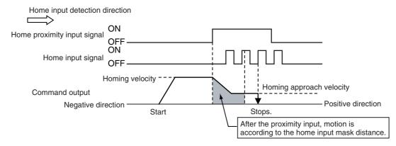
• If you start homing while the home proximity input signal is ON, the operation will start at the homing velocity in the direction opposite to the home input detection direction. After the home proximity input signal turns OFF, the homing operation will start at the homing approach velocity in the home input detection direction.
