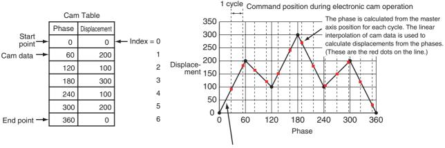
Linearly interpolate between cam data (black dots on the line).
