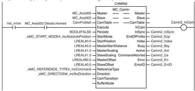
The MC\_CamIn (Start Cam Operation) instruction is executed for axis 4 (slave axis) if *Vel\_InVel* is TRUE for the MC\_MoveVelocity (Velocity Control) instruction and homing is completed for axis 4.
