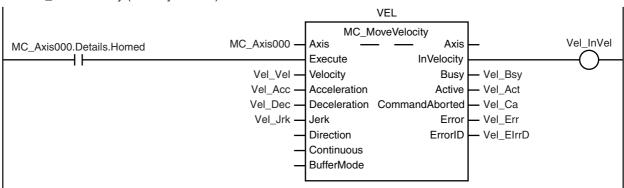
Latch processing is executed after the MC\_MoveVelocity (Velocity Control) instruction is started.
