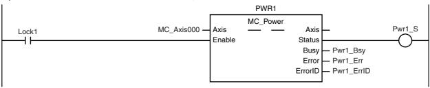
If process data communications are active for axis 2, the Servo is turned ON.
