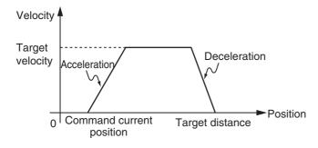
When the *Acceleration* (Acceleration Rate) or *Deceleration* (Deceleration Rate) is 0 and the instruction is executed, the axis will reach the target velocity without accelerating or decelerating. The following chart shows an operation example of when the acceleration rate is 0.
