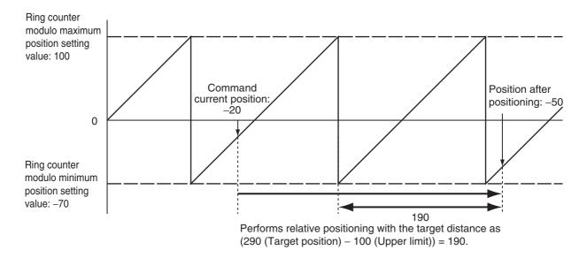
When the shortest way is specified for *Direction*, positioning starts in the direction with the shortest distance between the command current position and the target position. The following chart shows an operation example when positioning starts with a command position of 50 and moves toward –20.
