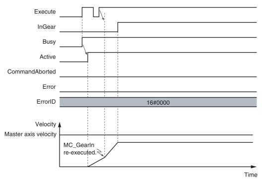
The following timing chart shows when the instruction is re-executed during the InGear phase to change the *RatioNumerator* (Gear Ratio Numerator) and *RatioDenominator* (Gear Ratio Denominator). The motion is the same as when *Acceleration* (Acceleration Rate) and *Deceleration* (Deceleration Rate) are both set to 0.
