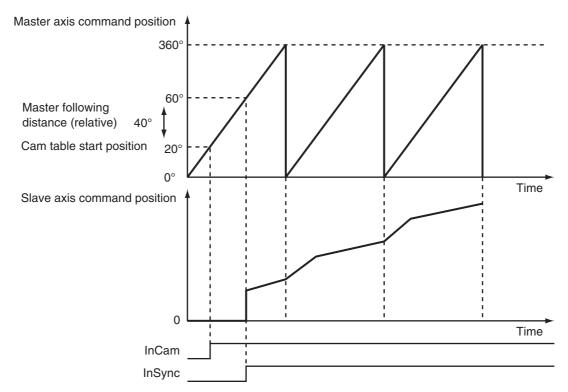
To specify the same operation in absolute coordinates, set the cam table start position to 20°, master start distance to 60°, Start Mode to absolute coordinates, and Execution Mode to Periodic.
