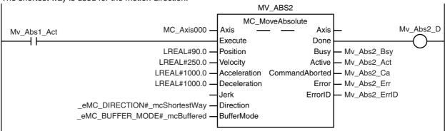
Absolute positioning 3 is executed with multi-execution of instructions to move from 90.0° to 120.0°. The shortest way is used for the motion direction.
