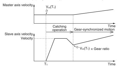
For the *Slave* (Slave Axis) to catch up with the *Master* (Master Axis) for the *MasterSyncPosition* (Master Sync Start Position) and *SlaveSyncPosition* (Slave Sync Start Position), the following condition must be met for the *Velocity* (Target Velocity)
