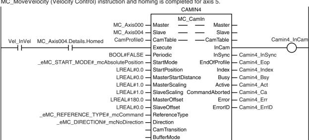
The MC\_CamIn (Start Cam Operation) instruction is executed for axis 5 (slave axis) if *Vel\_InVel* is TRUE for the MC\_MoveVelocity (Velocity Control) instruction and homing is completed for axis 5.
