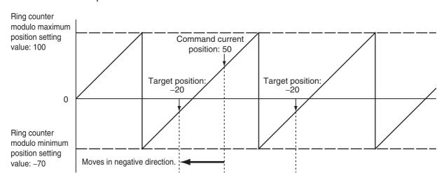
Positioning starts towards the target position within the ring counter range when No direction is specified for Direction. Therefore, the size relationship between the command current position and the target position determines the direction of travel.
