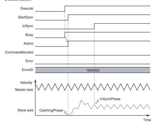
You can specify the *Acceleration* (Acceleration Rate) and *Deceleration* (Deceleration Rate) as input variables. The following figures show operation examples of the electronic gear.
