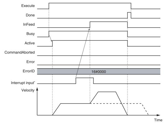
\* There may be a delay of up to several control periods from when the interrupt input turns ON until *InFeed* changes to TRUE.
