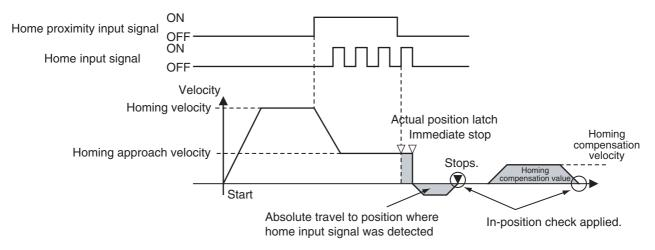
• Waiting for the in-position state is always performed for this instruction regardless of the setting of the In-position Check Time axis parameter.
