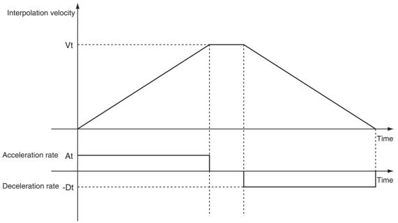
Vt: Specified interpolation velocity, At: Specified acceleration rate, Dt: Specified deceleration rate.
