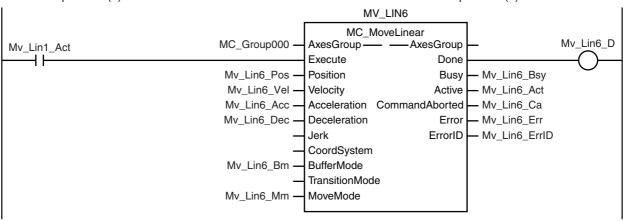
Linear interpolation (7) is executed with multi-execution of instructions after linear interpolation (1) is started.
