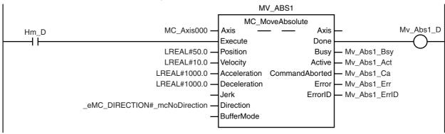
After absolute positioning 1 is started, absolute positioning 2 is started with multi-execution of instructions.
